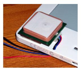
This unit was constructed in a similar way to my other Kobo Touch with a BlueFly vario module mounted internally
