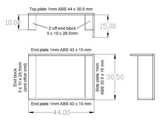
The corners were rounded and the cover fixed to the Kobo using thin double sided tape with two sides overhanging the corner of the Kobo. Glass reinforced tape was then applied externally as reinforcement.
