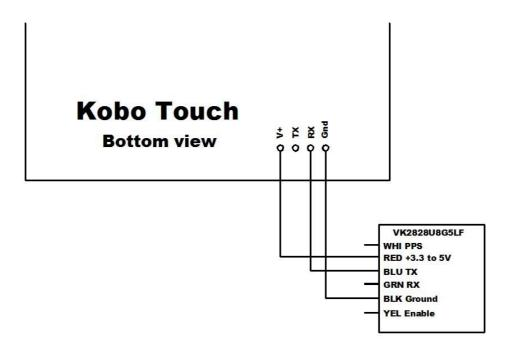
There is no facility for an external backup supply but the module appears to have some kind of internal capacitor backup system. The V.Kel datasheet does not suggest the use of external components as with the GlobalTop modules.
